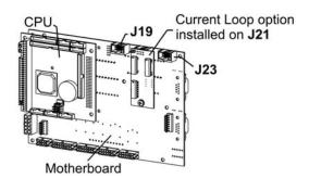
Example setup: install jumper shunts for voltage output on J19 and J23; remove jumper shunts and install Current Loop option for current output on J21.
